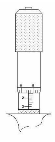
Figure 8. Slit Width Setting: 1380 Micrometers (1.38 mm)
